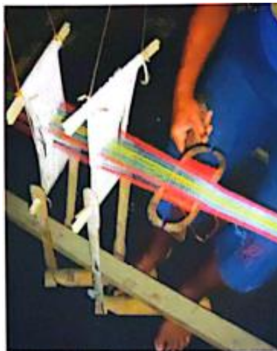
Figure 1. Loom used by Tabanan weavers to produce 10 cm wide bands
